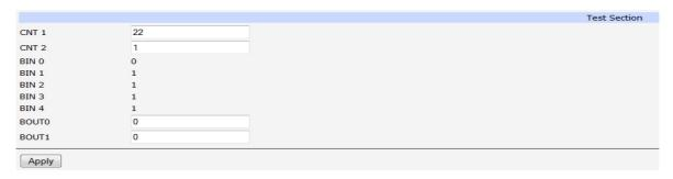
CNT X: For setting the counter inputs to specific values between 1 and 10. This allows you to make a quick first alarming test. Even without real drycontact-pulses from a PLC.
