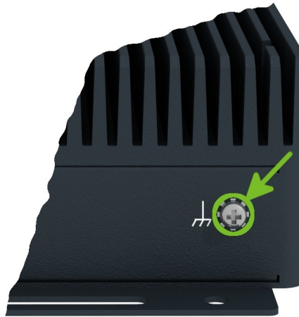
Figure 9: Position of the Grounding Screw
