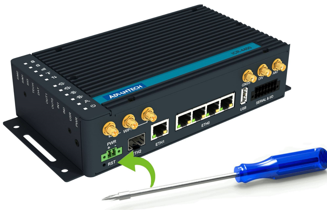
Figure 15: Resetting the Router
