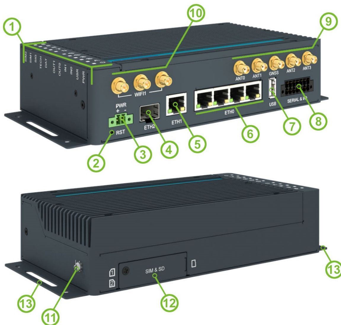
Figure 5: Hardware Overview of the Router
