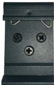
Figure 6: Default position of DIN rail clip
