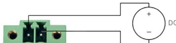
Figure 10: Connection of power supply
