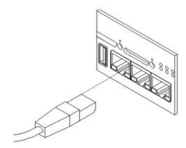
Figure 26: PORT1 cable connection
