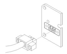
Figure 30: Connection of I/O cable
