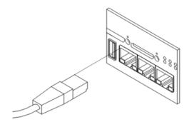
Figure 27: PORT2 cable connection
