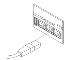
Figure 25: Connection of ethernet cable
