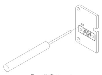
Figure 32: Router reset
