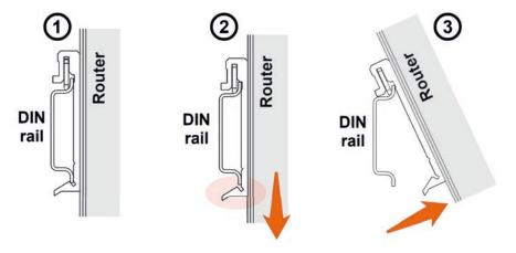
Figure 18: Removal from the DIN rail
