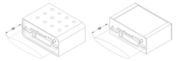
Figure 15: Space in front of connectors (plastic) Figure 16: Space in front of connectors (metal)
