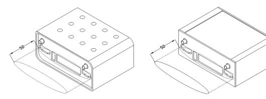
Figure 15: Space in front of connectors (plastic) Figure 16: Space in front of connectors (metal)
