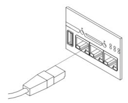
Figure 26: PORT1 cable connection
