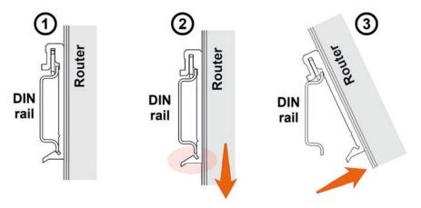
Figure 18: Removal from the DIN rail
