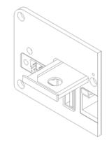
Figure 23: Ejected SIM holder
