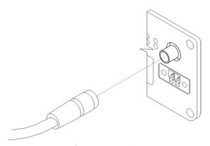
Figure 22: Connecting of the antenna
