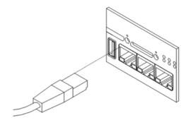
Figure 27: PORT2 cable connection
