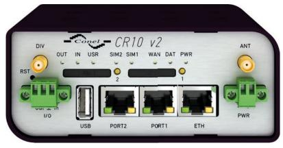
Figure 19: Front panel CR10 v2F
