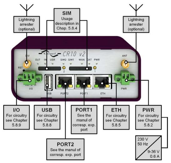
Figure 33: Router connection
